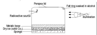
From the diagram above the base of the chamber is maintained at about -80°C and the top is at room temperature so that there is a temperature gradient between the <u>top and bottom</u>.
